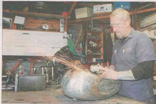
GRINDING. Renwick's Tony Hodgson works on fuel tank for a 1957 Triumph 650 Thunderbird he is rebuilding. Photo: Blair Emmer 167567
